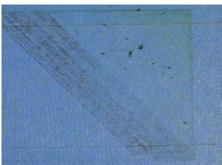
Nozzle and heated bed too close in distance
