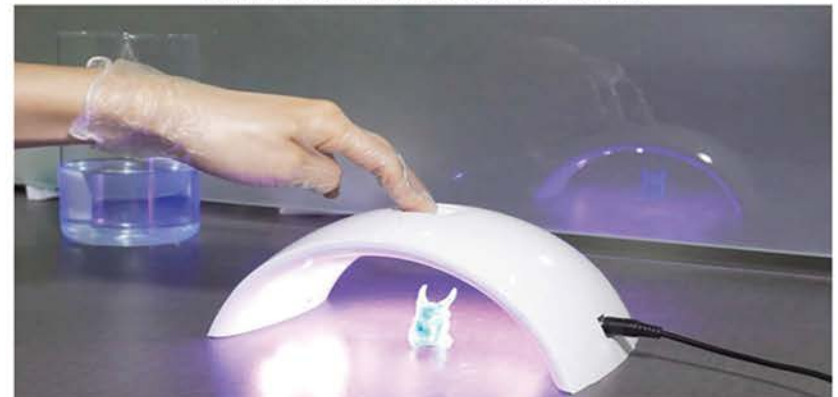
Step14: Irradiate the model with UV-light about 2-3mins.
