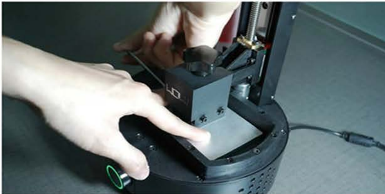
Step6: Press down the platform and tighten the four screws on both sides of the platform.
