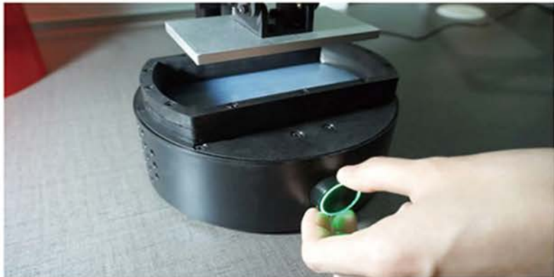
Step5: Rotate the knob drops the platform to the lowest point.
