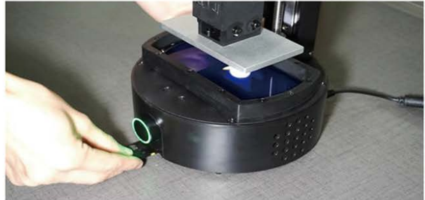
Step8: Insert the SD card into the slot (Face down).
