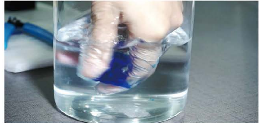
Step13: Clean the model with 99% alcohol.
