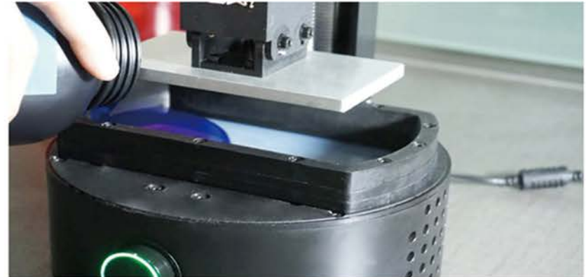
Step7: Pour the resin into resin tank(Less than 120g resin).
